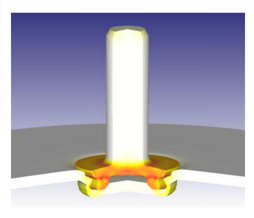
A pull test is shown after installation of a self-clinching fastener. In this case, the force predicted by DEFORM™ was within 10% of the experimental value. This demonstrates a powerful multiple deforming body capability for large deformation.
