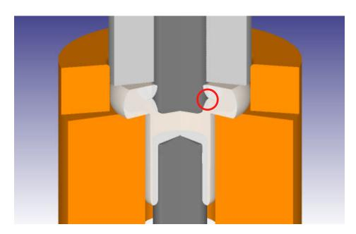
A fastener lap is shown during the final operation of a cold formed automotive part.
