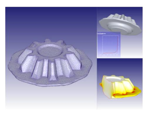
DEFORM-3D includes a very sophisticated postprocessor. Over and above the multiple document interface (MDI), each postprocessing session is capable of displaying up to six coupled viewports. The mesh, shape, load-stroke curve, effective strain and sliced section of the workpiece are displayed in the above illustration. It is easy to compare two simulations with slightly different parameters.
