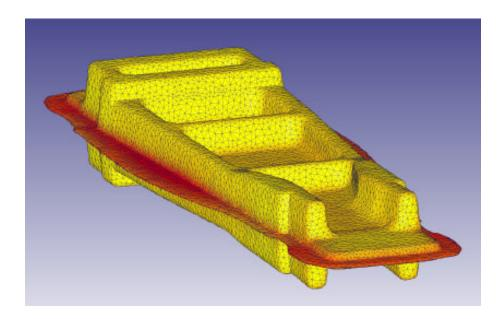
The automatic mesh generator (AMG) produces an optimized mesh system with local element size control based on the specific process being analyzed. This facilitates the enhanced resolution of part features while maintaining good control of the overall problem size and computing requirements. A user-defined local mesh density provides advanced users a flexible control to meet their requirements.
