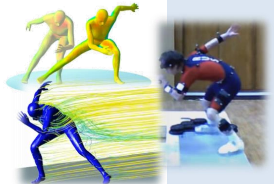
Figure 7: Aerodynamics of skating. The body motion is defined via motion capture.
